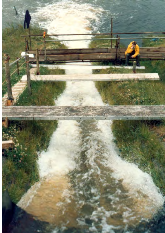
GRASSCRETE under test with tail water observation
