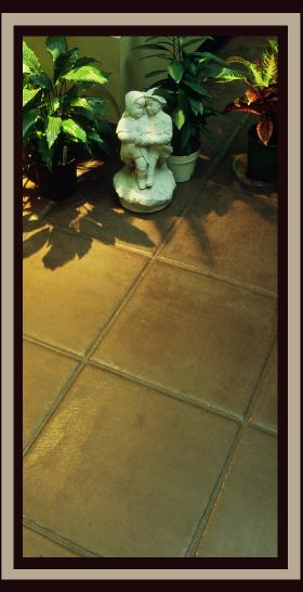
The Bomanite 12" x 12" Tile pattern is imprinted without texture and has a smooth surface between the joint lines, resembling porcelain or ceramic tile. Bomanite patterns are the original cast-in-place, colored and imprinted architectural concrete paving.
